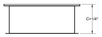
\*NOTE: 1/4" ADDER REQUIRED TO ACCOUNT FOR THICKNESS OF COVER
