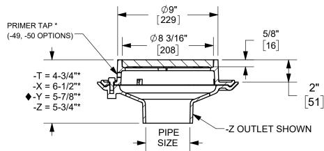
$^{\star}$  FOR TRAP PRIMER CONNECTION BELOW DRAIN, USE 88400 OR 88450 ADAPTER.
