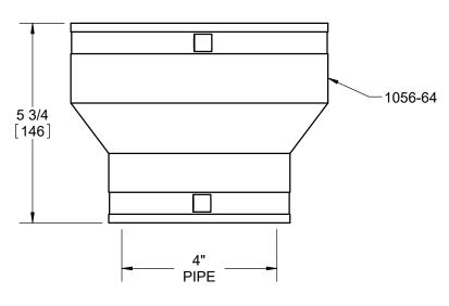
\*MAX. SERVICE TEMPERATURE OF RUBBER REDUCER REMAINS 140°F
