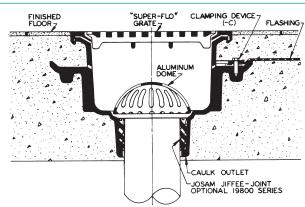
49320A-NB Series SUPER-FLO-SEPTOR  $^{\circ}$  Floor Sink shown installed in a heavy-duty structural concrete finish floor.
