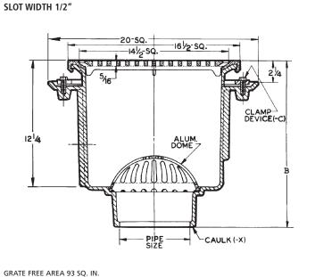
TYPE NO. PIPE SIZE B DIM. LBS. 49423-NB 15-1/2 128 3 49424-NB 4 15-3/4 129 49426-NB 6 16-1/4 132 49420-LF-NB SERIES
