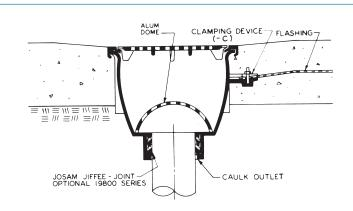
49580A-NB Series SUPER-FLO-SEPTOR  $^{\otimes}$  Floor Sink shown installed in a poured concrete floor on the ground level.
