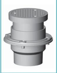
55000-Y Series KLEENATRON® Cleanouts feature JOSAM JIFFEE-SET connections with MULTI-TITE® service weight (SV) soil pipe gaskets in 2, 3 and 4 inch sizes for labor-saving assembly to service weight and no-hub cast iron pipe, and to PVC and ABS pipe. Merely lubricate gasket and pipe, set cleanout in place, push down until top of pipe contacts built-in stop and the joint is complete.
